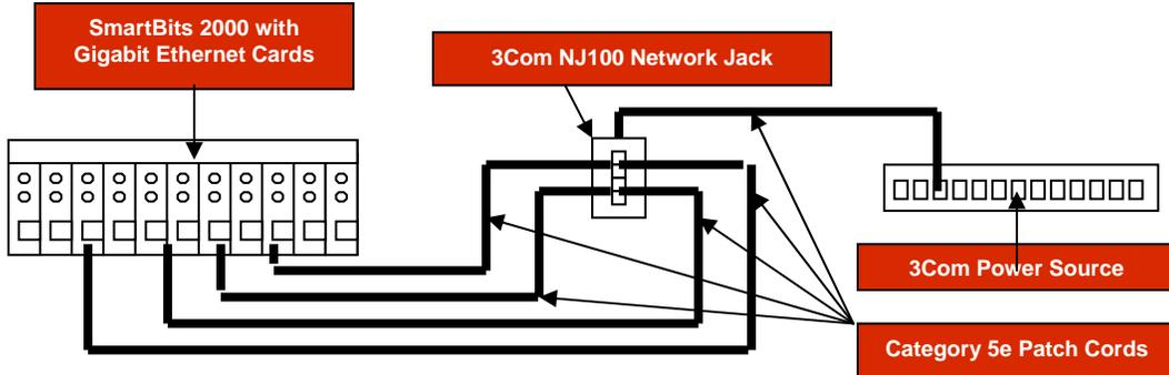
Figure 2: Utilizing the NJ100 for a local connection
