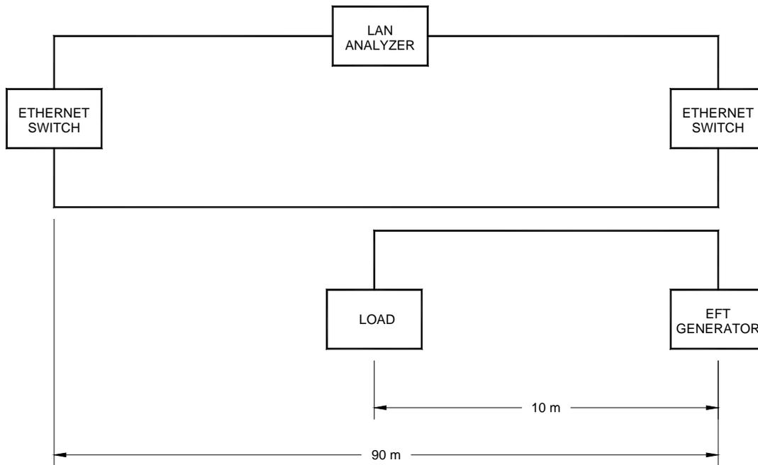
**Figure 1:** EFT noise immunity test setup
