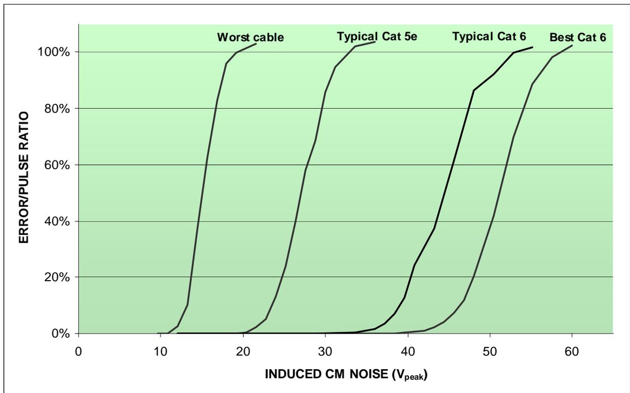
**Figure 4:** EFT noise susceptibility measurements
