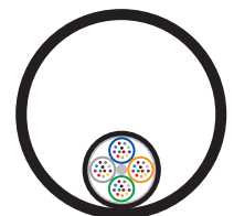
48-count loose tube fiber cable in a traditional plenum innerduct (1.0 in. ID)
