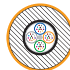
48-count loose tube fiber with Berk-Tek Armor-Tek (.712 in. OD)
