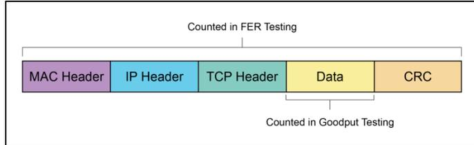
Figure 1: Ethernet Frame Components
